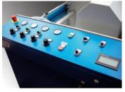
The easy to use plc controls incorporate a modem link for remote diagnostics. Pneumatic operation of all rollers allow differing pressures on nip and pull rollers. Individual temperature adjustment of all rollers facilitate the use of specialist films.
