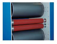
Large 260mm diameter Teflon coated pre-heat rollers and 75mm heated nip rollers with an advanced rubber compound give maximum heat transfer for high speed, scratch free results.
