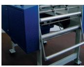
A bail arm regulates the speed of the cutter and allows it to keep pace with the encapsulator.
