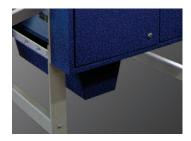
An electrically interlocked catch tray is incorporated to collect trim waste which doubles as a guard for the lower blade as the cutter will only operate when the tray is in position.
