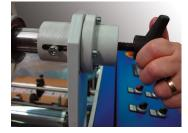
The madrel has a hinged support and film can be adjusted laterally on the run to minimise waste and down time.
