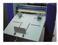
The adjustable burster automatically separates sheets. A cushion of air supports the sheet as it is delivered into the catch tray.
