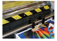
An infeed roller presents lightweight and digital output to the laminating and nip rollers where a no sheet detector helps to prevent unwanted wraparounds.
