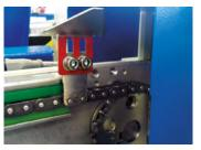
The flying knife separator has two specially designed chain driven blades to separate, nylon, polyester and OPP up to 75 micron.
