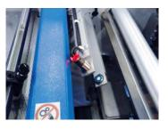
A sensor detects the underlap for accurate separation.
