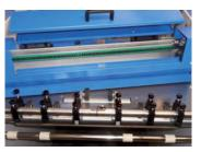
A cushion of air supports the sheet as it is delivered into the catch tray.
