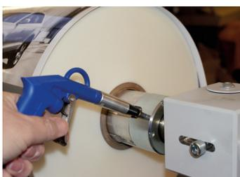
The film mandrel swings out and has an air shaft to speed roll changes. The film can be adjusted laterally on the run to minimise waste and down time.
