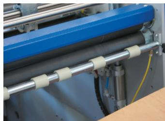
The adjustable burster automatically separates sheets up to B2 size. A cushion of air supports the sheet as it is delivered into the jogger.
