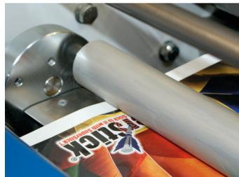
A decurl bar, which may be altered on the run, is fitted to assist in giving a flat result.
