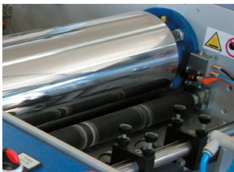
A pneumatically controlled infeed roller presents lightweight and digital output to the laminating and nip rollers where a missing sheet detector helps to prevent unwanted wraparounds.
