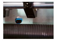
A pneumatically controlled infeed roller presents lightweight and digital output to the laminating and nip rollers where a no sheet detector helps to prevent unwanted wraparounds.
