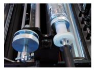
Film can be adjusted laterally on the run to minimise waste and down time.
