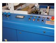
The centralised PLC control panel offers ease of operation and is enhanced with a modem link for remote diagnostics.
