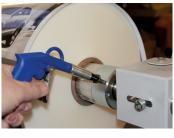
The film mandrel swings out and incorporates an air shaft to speed roll changes.
