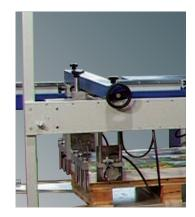
Sheet size changes are easily accommodated as two rear paddles and sheet stops may be moved in one operation using the wheel on the operator's side of the stacker.
