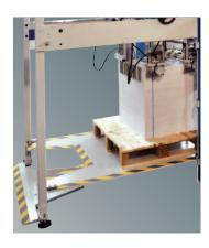
The stacker table lowers all the way to the floor for easy removal of the pallet.
