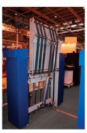
The infeed table is pneumatically lifted and lowered to allow good access for webbing and for maintenance to the rear of the laminator.
