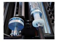
The film mandrel swings out and incorporates an air shaft to speed roll changes.
