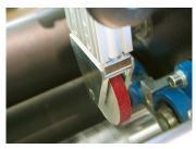
The positioning of the pneumatically controlled perforator overcomes any potential issues caused by poor film roll profiles allowing higher speeds to be maintained.
