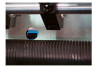
An pneumatically controlled infeed roller presents lightweight and digital output to the laminating and nip rollers where a no sheet detector helps to prevent unwanted wraparounds.
