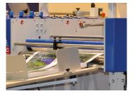
The adjustable burster automatically separates sheets up to B1 size whilst a blower bar provides a cushion of air to support the sheet as it is delivered into the Jogger.
