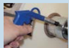
Expanding film mandrel for quicker film changes.
